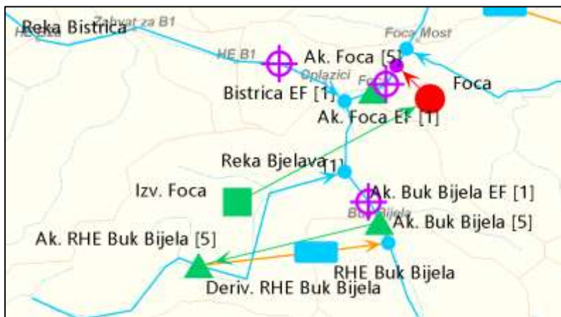
Figure 3-6: Representation of the pumped-storage HPP Buk Bijela in the Drina WRM model.
